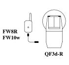
In Wireless Auto Fill, the Qflash will track the camera settings automatically and use it's built in light sensor to control exposure. The Fill ratio dial on the QTTL adapter can be used to fine tune exposure.
