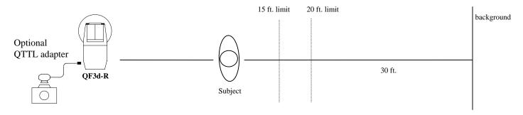
By limiting the sensor distance, the sensor will focus only on the subjects that are within the sensor limit. It will no longer try to balance the light from a far background and near subject.
