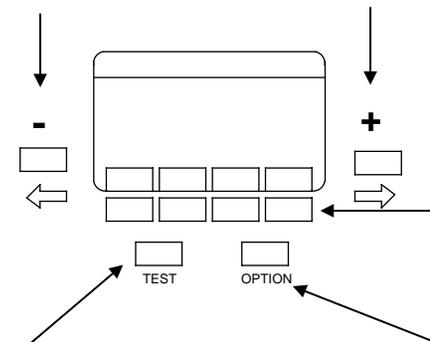
The **TEST** button will fire the remote flashes. An option allows you to choose whether the remotes fire all at once, or sequentially so you can test individual exposures.
