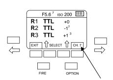
Set the channel code on the *PILOT* to the same as the FW8R (See Section 3.4 of *PILOT* instructions.)
