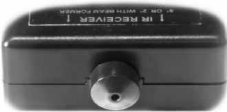
2° baffle in place
