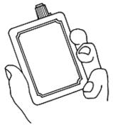
Pull up knob. Do not squeeze front panel, otherwise switch mechanism will be difficult to operate.
