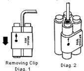
When replacing the clip, snap it onto the module as shown (diag. 2). The red marker on the clip should point to the red marker on the module.
