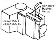
Place one adhesive backed piece of Velcro on the flash and the other on the Locking Plate (provided with the module).
