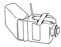
Secure the battery door with the velcro strips provided with the module. Place one adhesive backed piece on either side of the battery door. Use the 4" long (10cm) piece to secure the door.
