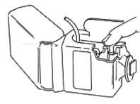
Press the module down inside the battery compartment until the lever springs back locking the module into place.
