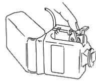
Push the module lever forward and insert the module into the battery compartment.
