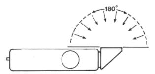
For darkroom measurements the white image plate should be parallel to the easel.
