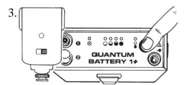
Turn the QB1+ ON. *Note: The QB1*+ *will not turn on until a module plug is connected.*
