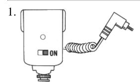
Connect the module to the flash. (See Module Instructions to explain the proper module position.) Turn the flash on.
