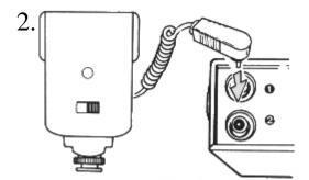
Plug the module into either one of the two flash output jacks on the QB1+.
