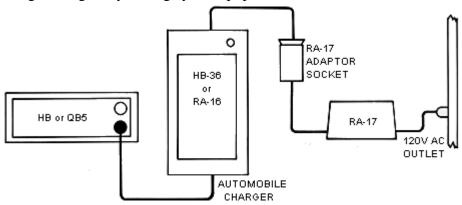
**IMPORTANT!** Make all connections before plugging the RA-17 into the AC outlet. After charging, always remove the RA-17 plug from the AC outlet first.
