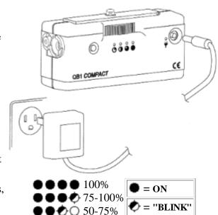
**2.9 Do not use a Bantam Battery charger.** A Bantam charger will not charge QB1c.
