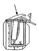
Lower the battery door. Slide Power Module T forward to lock into place.
