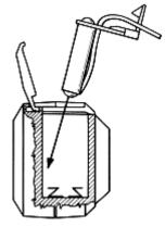
Insert Power Module T with the ends of the post towards the rear of the Battery Chamber.
