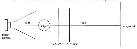
By limiting the sensor distance, the sensor will focus only on the subjects that are *within* the sensor limit. It will no longer try to balance the light from a far background and near subject.
